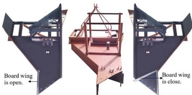
Figure 7. Open and close of board wing for the machine tail to prepare the soil surface in the form of flat or ridges.
